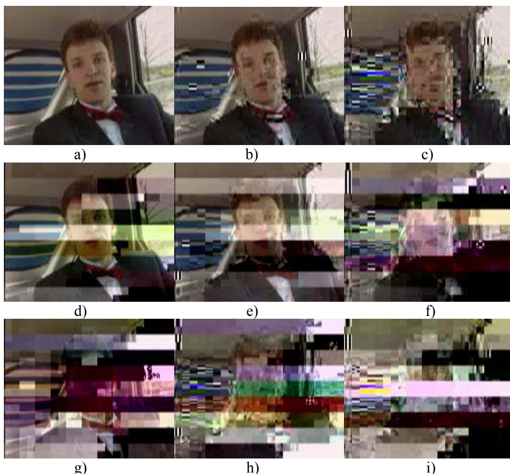
Fig. 1 The encryption results of the 1st frame in “Carphone”: a) (p_{sr}, p_{sd}) = (0, 0) – the plain frame; b) (p_{sr}, p_{sd}) = (0, 0.2) ; c) (p_{sr}, p_{sd}) = (0, 1) ; d) (p_{sr}, p_{sd}) = (0.2, 0) ; e) (p_{sr}, p_{sd}) = (0.2, 0.2) ; f) (p_{sr}, p_{sd}) = (0.5, 0.5) ; g) (p_{sr}, p_{sd}) = (1, 0) ; h) (p_{sr}, p_{sd}) = (1, 0.2) ; i) (p_{sr}, p_{sd}) = (1, 1) .
